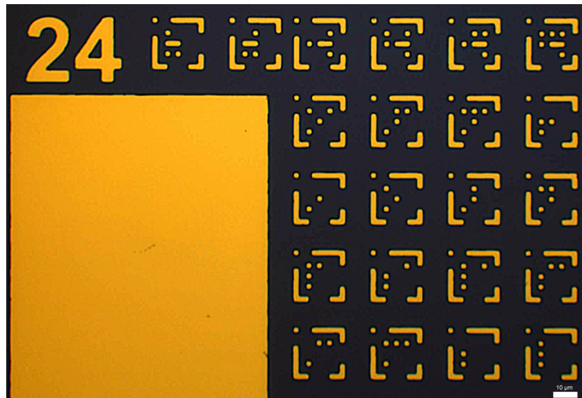
Figure 2–8: Patterns after lift-off ("AFM-friendly" mask, part). The golden part is the metal pattern while the dark part is the substrate. The resolution is \sim 2.0 \mu\text{m} , slightly smaller than after the development. Scale bar is 10 \mu\text{m} .
